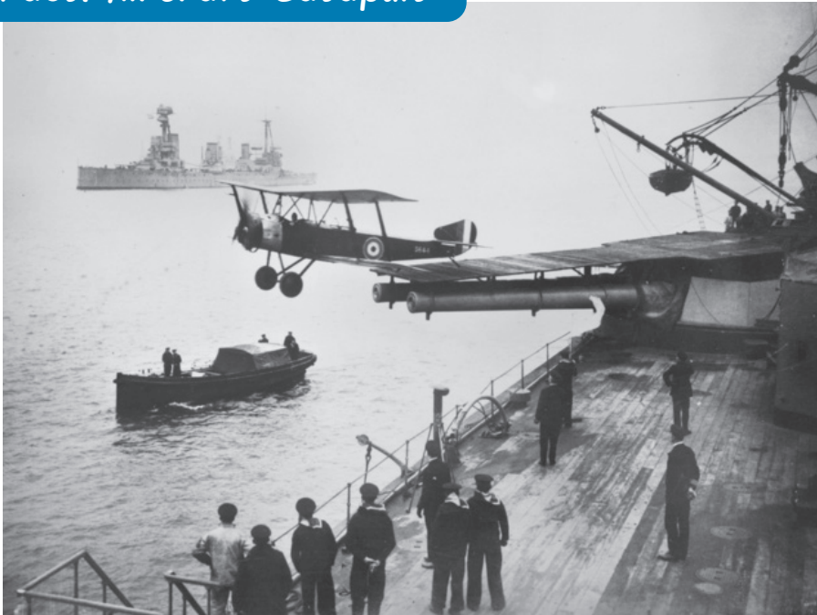
In the North Sea on 4 April 1918, and again on 11 May 1918, 5644 Sopwith 1 1/2 Strutter successfully took off from HMAS Australia with two crew and wireless equipment. This had not been previously done with a two seater aircraft.
