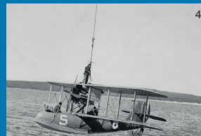
3. 9 Squadron plane taxiing towards HMAS Australia . A member of the aircrew is climbing onto the mainplane to attach the crane cable when the plane is stationary. Australia's life boat is about to be lowered to retrieve the aircrew. Unknown photographer About 1942 Reproduction of a black and white photographic print Collection of the Australian War Memorial P05536.001
