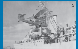
5. A2-7 Supermarine Seagull V being craned aboard what is most likely to be HMAS Hobart . The catapult will be extended, the plane repositioned on it and secured. Unknown maker About 1939 Reproduction from a black and white photographic negative Collection of the Australian War Memorial 044445
